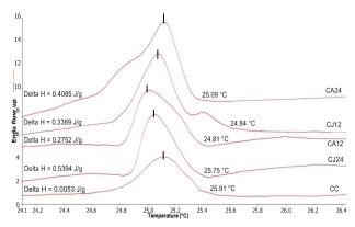
Figure 2. DSC thermal transition curve of commercial collagen (CC) and threadfin bream collagens extracted using calamansi juice (CJ) and 0.5M citric acid (CA) for 12 and 24 hrs
