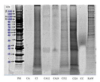
Figure 4. SDS-PAGE pattern of threadfin bream collagens, commercial collagen and raw threadfin bream. From left protein marker (PM), citric acid (CA), calamansi juice (CJ), citric acid 12 hrs collagen (CA12), citric acid 24 hrs collagen (CA24), calamansi juice 12 hrs collagen (CJ12), calamansi juice 24 hrs collagen (CJ24), commercial collagen (CC) and threadfin bream waste (RAW)
